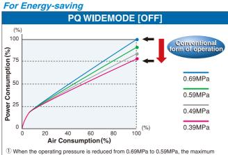
power consumption is automatically reduced to about 92% of 0.69MPa. 2 When the pressure is reduced to 0.49MPa, the power consumption reaches about
