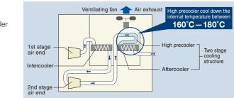
DSP series can not run in excess of 40°C of ambient temperature. Ventilation and/or air conditions should be considered to maintain the compressor room temperature.
